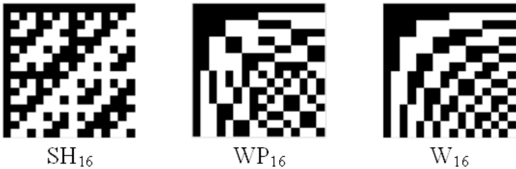
Figure 3.12 Binary display of Sylvester type, Walsh-Paley, and Walsh Matrices of size 16x16.
