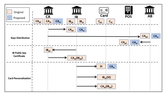
Figure 6-1: The Keys Distribution in the Proposed Scheme
