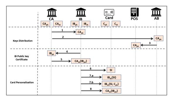
Figure 4-1: Keys Distribution, IB public key certificate and Personalisation processing in the EMV Card Authentication Methods
