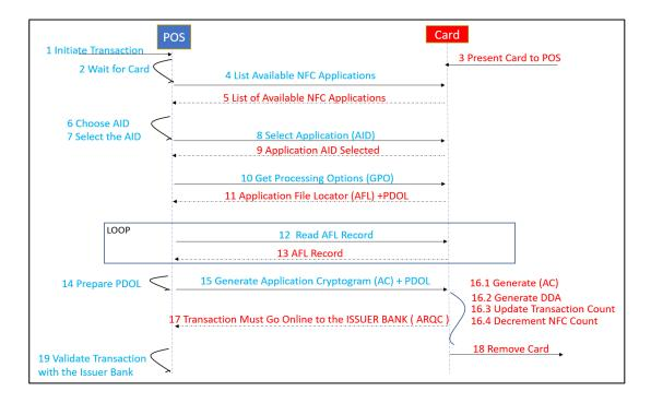
Figure 2-5: EMV Contactless Card Online Transaction Sequences
