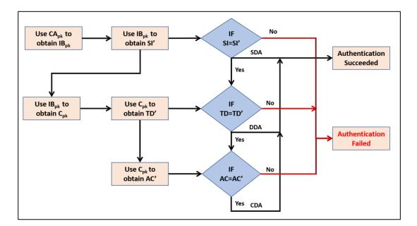
Figure 4-3: Authentication stage of the SDA, DDA, and CDA
