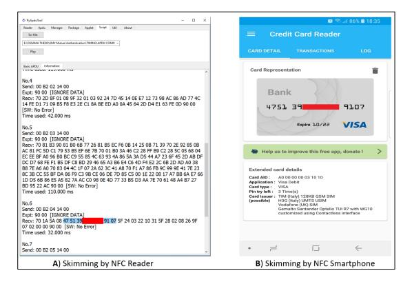
Figure 2-7: Examples of Skimming Attack by both NFC Reader & Smartphone Relay Attack
