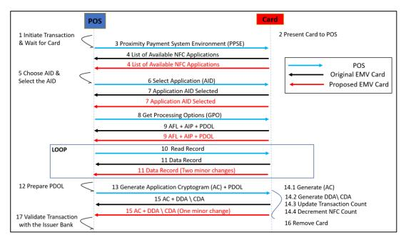
Figure 5-5: Original VS. Tokenisation EMV Transaction Phase
