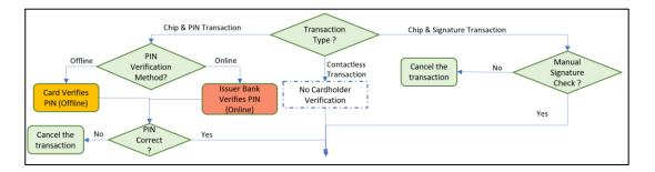
Figure 2-3: EMV Cardholder Verification Methods (CVM)
