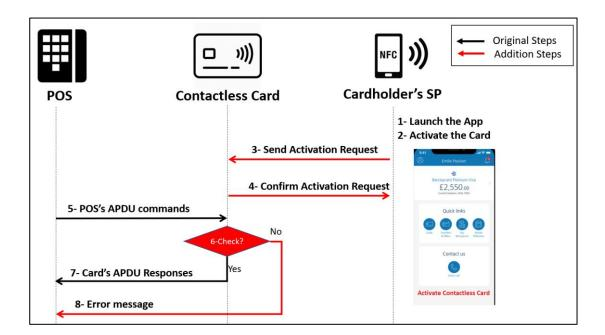
Figure 8-1: NFC Smartphone to Control the EMV Contactless Cards Proposed Scheme
