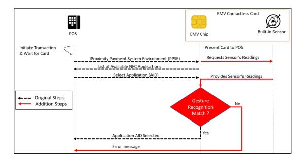
Figure 7-1: Gesture Recognition Based Proposed Solution for the EMV Contactless Cards
