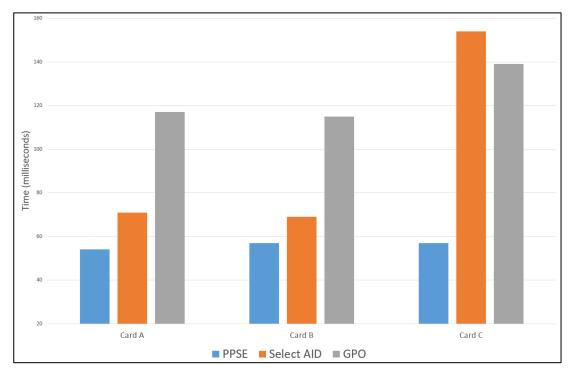
Figure 6-4: Timing Results for the Mutual Authentication scheme
