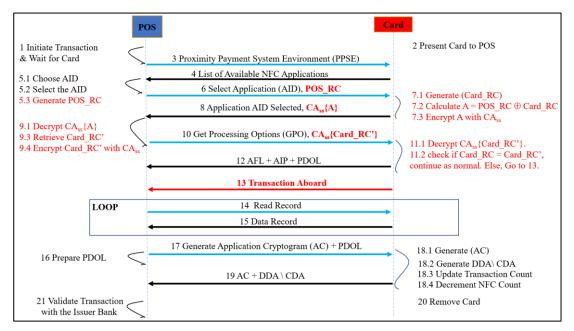
Figure 6-2: Transaction Phase in the Proposed Scheme
