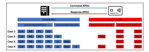
Figure 3-1: APDU Command & Response Structure
