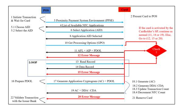
Figure 8-3: The Proposed Scheme in the Transaction Phase
