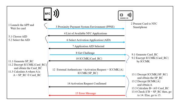
Figure 8-2: The Proposed Scheme in the Activation Phase
