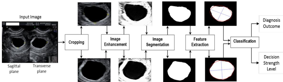
Figure 2: Block Diagram of the Major Steps of the Proposed Method
